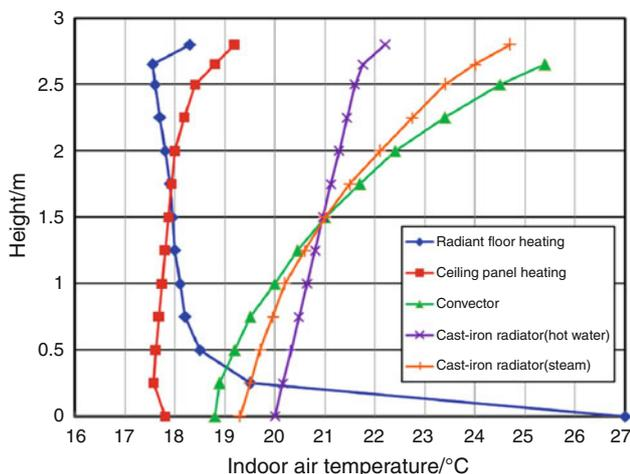
**Fig. 2** Comparison of indoor temperature distribution on heating systems
