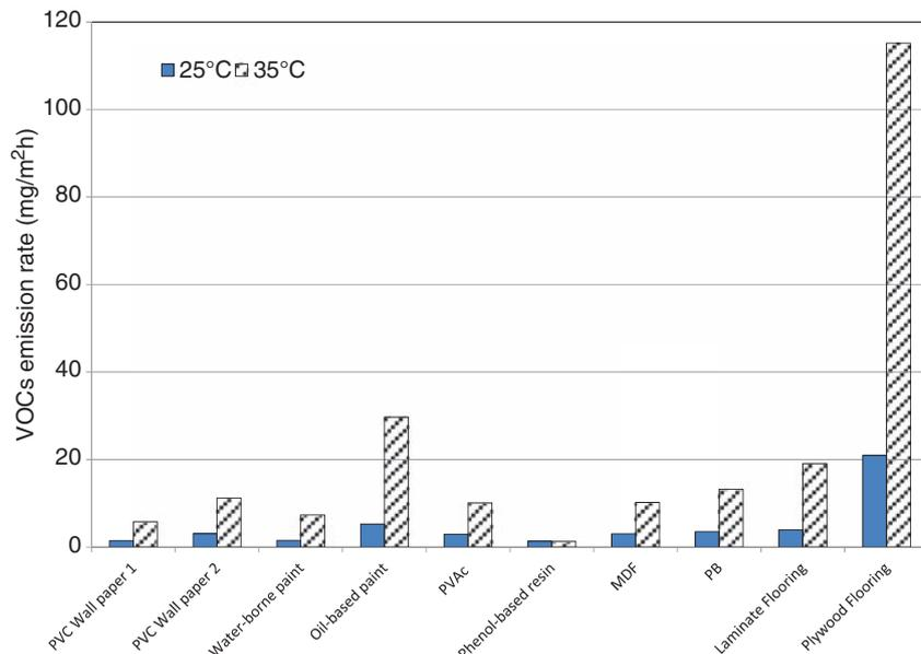
**Fig. 4.** VOCs emission rate from building materials according to temperature variation.
