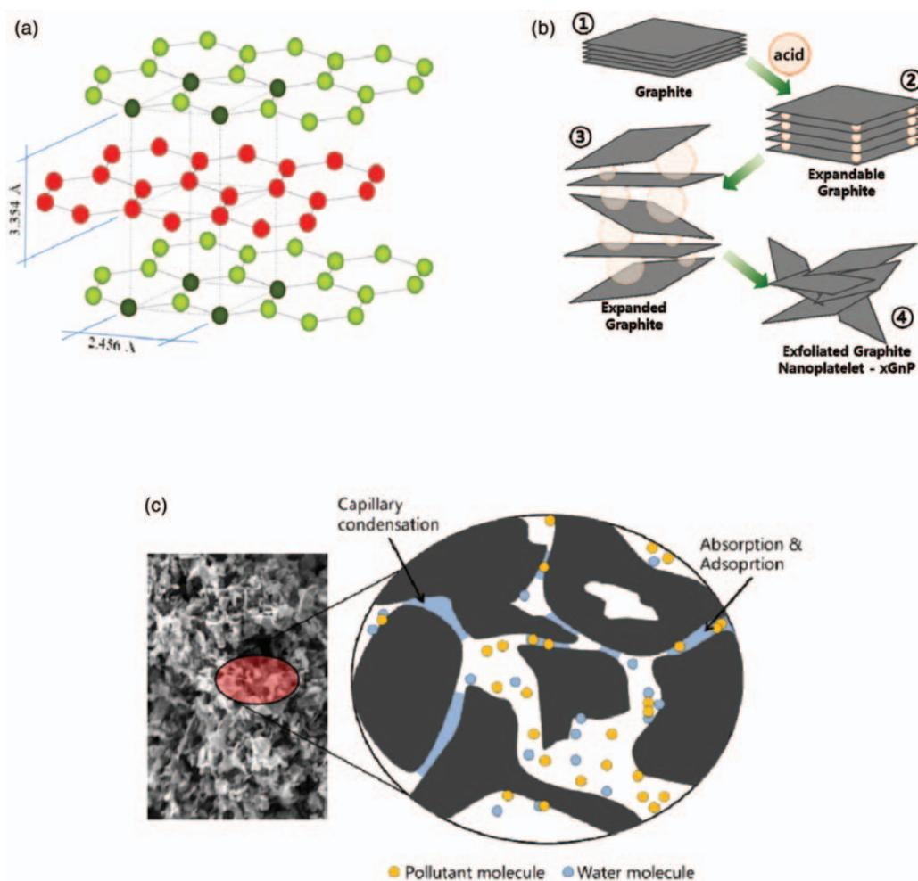
**Fig. 6.** Improved capacity of adsorption/absorption in porous media: (a) structure of graphite; (b) expansion and exfoliation process of xGnP; (c) water vapour effect on contaminant adsorption/absorption in porous media.
