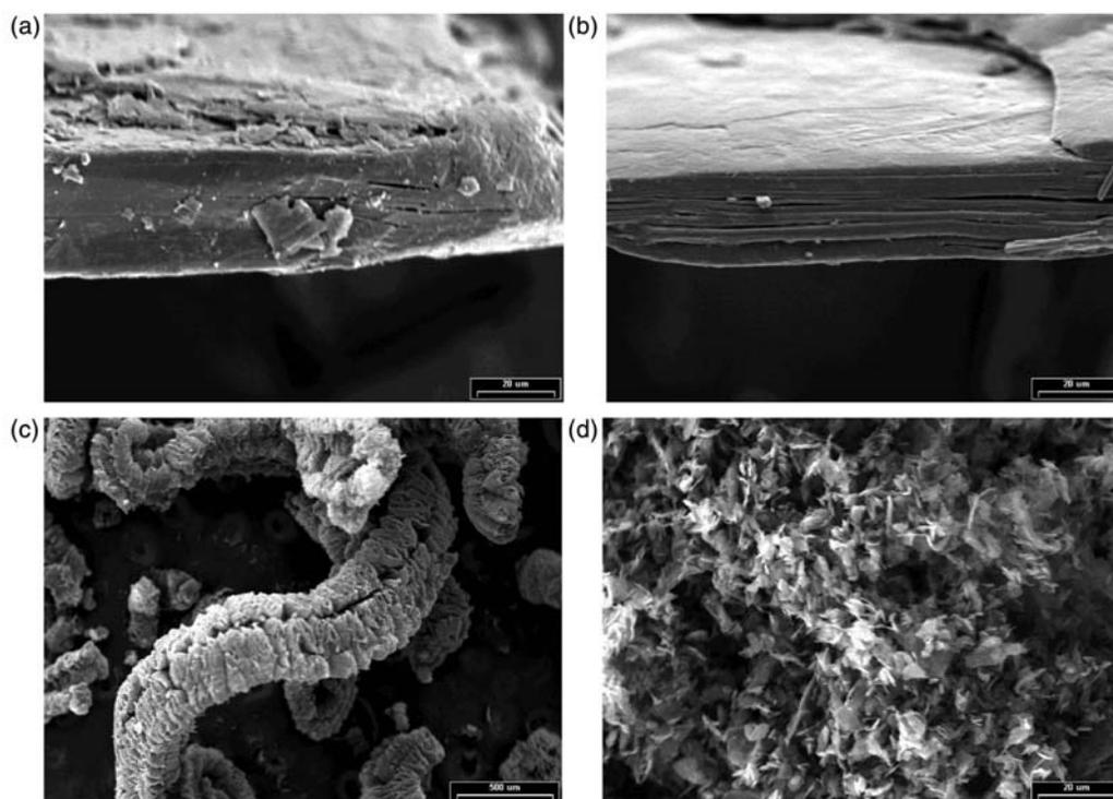
**Fig. 2.** Morphological changes of graphite according to the modifying process: (a) natural graphite; (b) expandable graphite; (c) expanded graphite; (d) xGnP.
