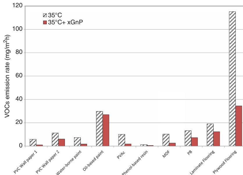
**Fig. 5.** The variation of VOCs emission rate according to the addition of the absorbent material.
