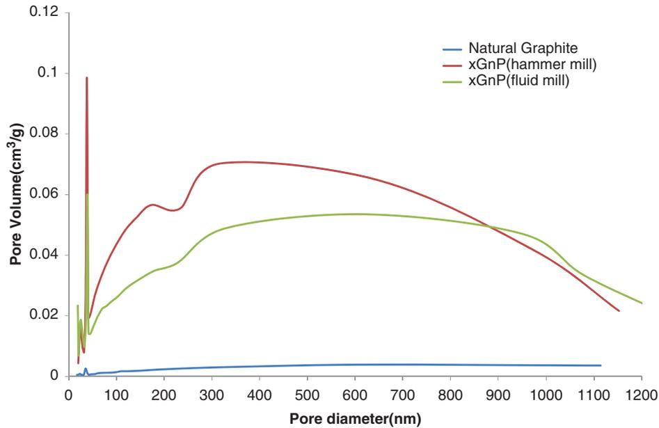
**Fig. 3.** Dispersion of pore volume and diameter of natural graphite and xGnP.
