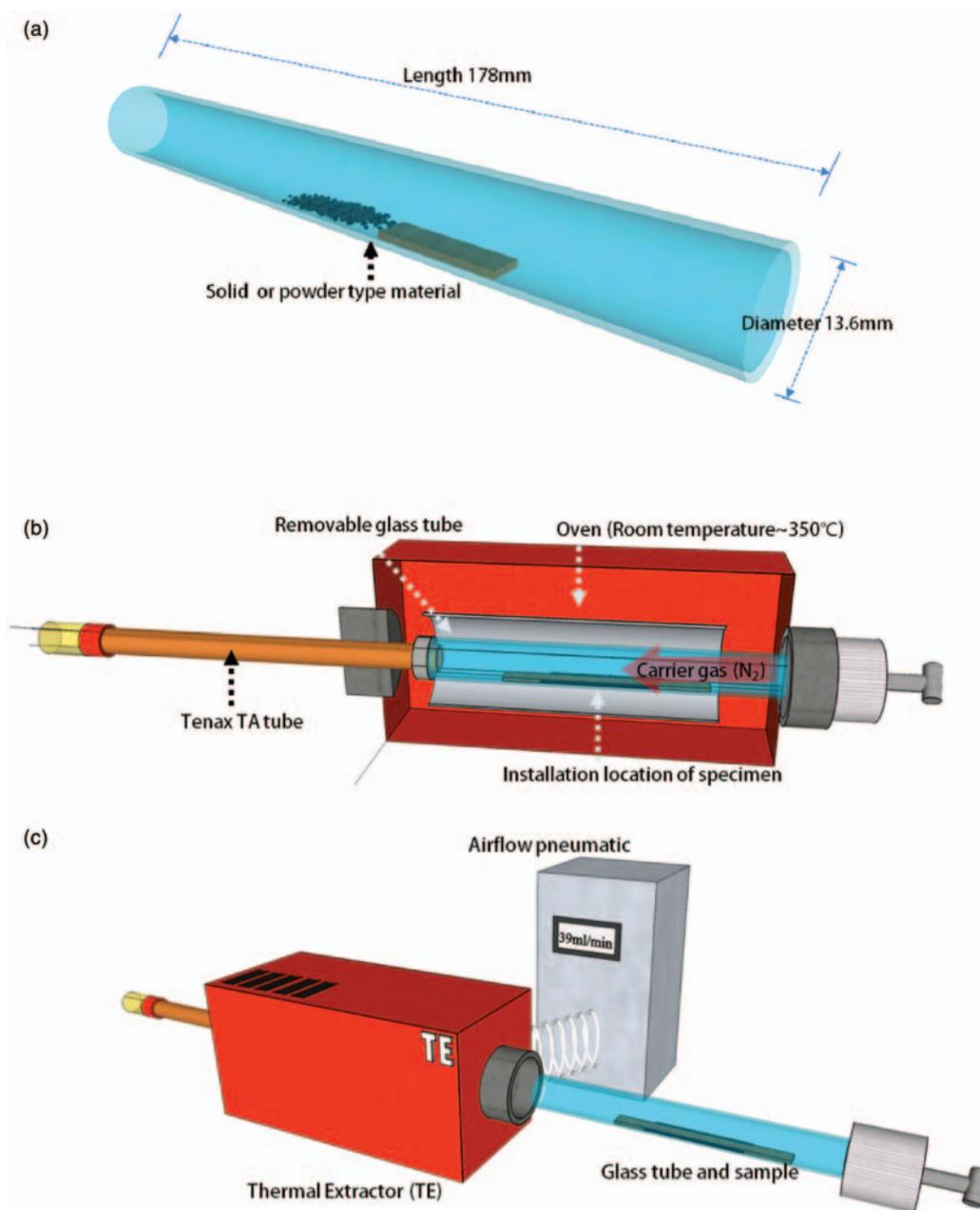
**Fig. 1.** Schematic diagram of the thermal extractor (TE): (a) glass tube and installation of specimen; (b) inner structure of TE; (c) the composition of the TE analysis apparatus.
