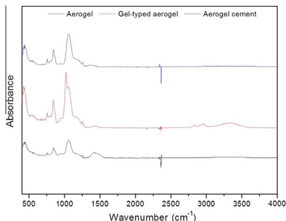
Fig. 4. FT-IR spectroscopy of each type of aerogel.
