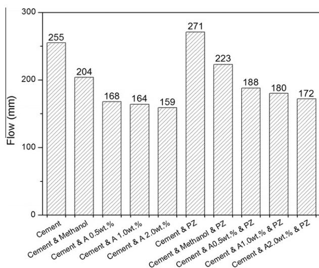
Fig. 9. Flow of fresh aerogel mortar.
