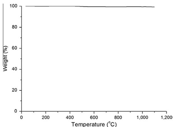
Fig. 3. TGA of silica aerogel (10 °C/min).
