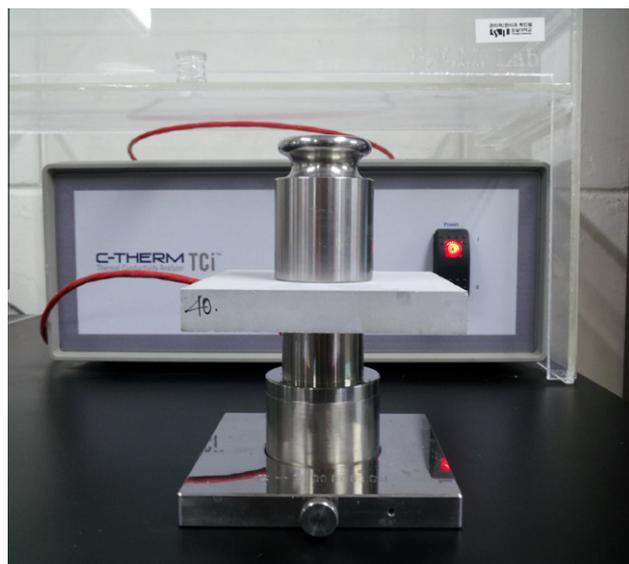
Fig. 2. Thermal conductivity analyzer (TCi).
