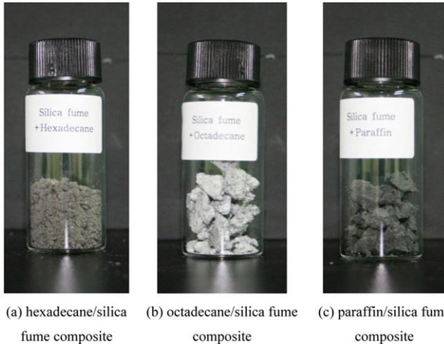
**Fig. 2.** Sample images of PCM/silica fume composites: (a) hexadecane/silica fume composite, (b) octadecane/silica fume composite, and (c) paraffin/silica fume composite.
