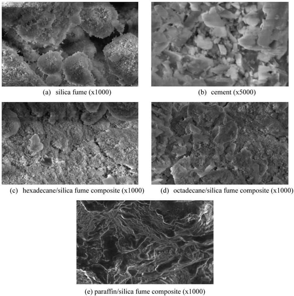
**Fig. 3.** SEM analysis of PCM/silica fume composites: (a) silica fume, (b) cement, (c) hexadecane/silica fume composite, (d) octadecane/silica fume composite, and (e) paraffin/silica fume composite.
