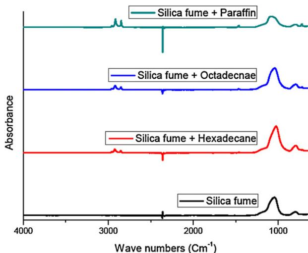
Fig. 4. FTIR analysis of PCM/silica fume composites.
