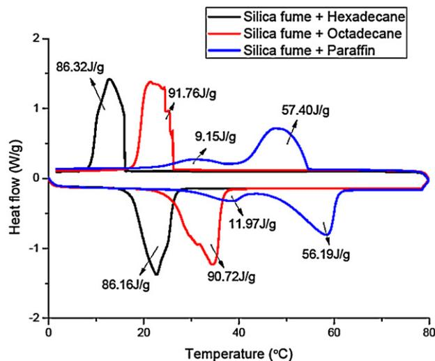
Fig. 5. DSC analysis of PCM/silica fume composites.
