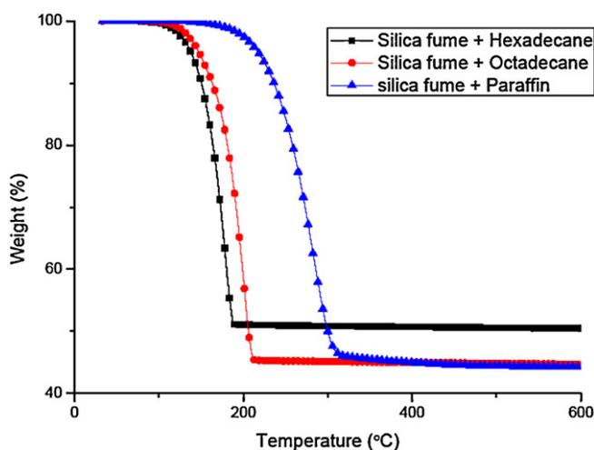
**Fig. 6.** Thermal gravimetric analysis of PCM/silica fume composites.
