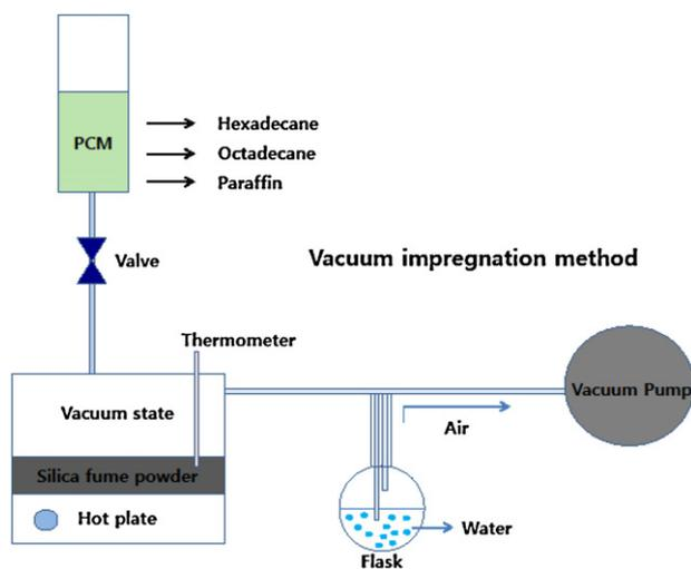
**Fig. 1.** A schematic of the vacuum impregnation method.
