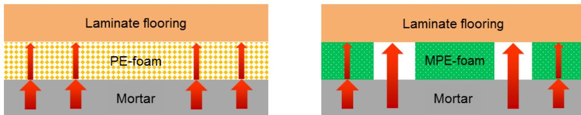
**Fig. 3.** Comparison of the heat transfer method between the PE foam and MPE foam
