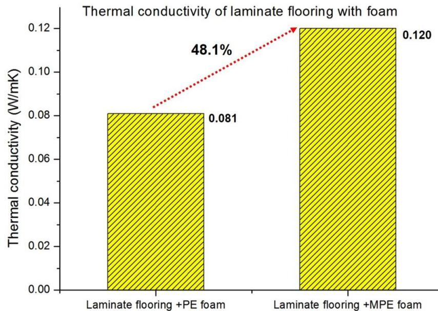
Fig. 4. Thermal conductivity of laminate flooring with PE foam
