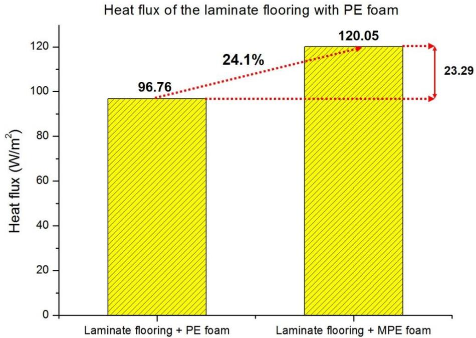
**Fig. 5.** Heat flux of the laminate flooring with PE foam
