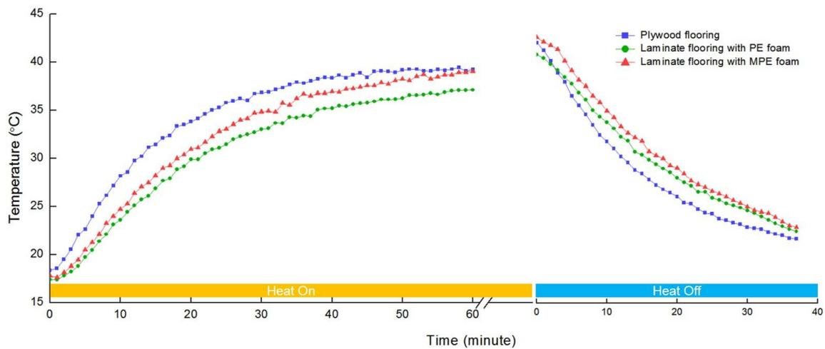
**Fig. 6.** Thermal transfer and latent heat performance of laminate flooring with PE foam and engineered wood flooring
