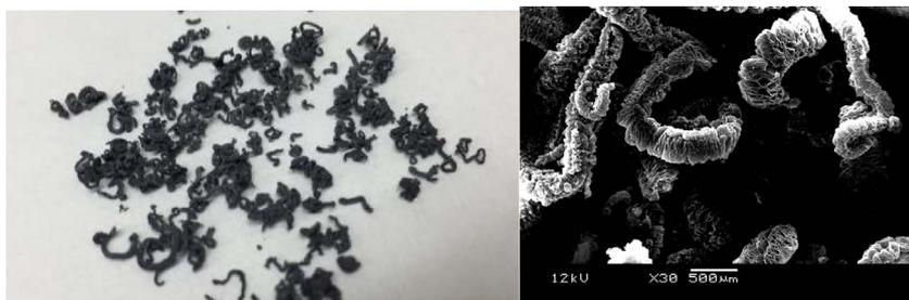
Fig. 1. Expanded Graphite.
